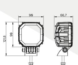
The BLUE Prime is designed to increase the efficiency of boom sprayer work in dark, in fog and during low visibility. The innovative construction is using polycarbonate, crystal LED lenses that generate strong and long blue light beam. The lighting provides excellent visibility along the entire length of the boom sprayer.
